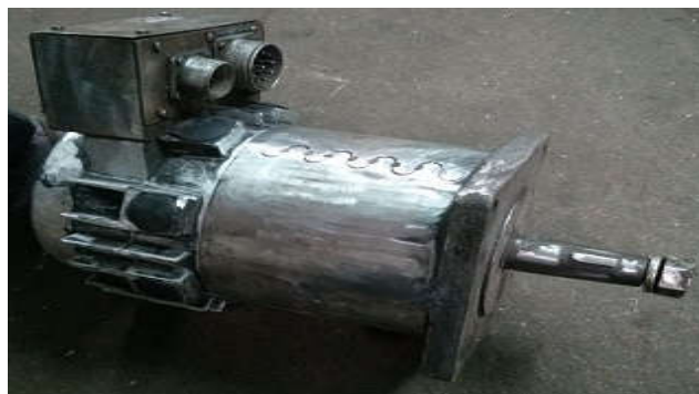
Fig 1 Photograph of PMDC Motor
