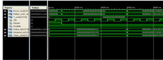
Fig 7: Simulation result of conventional adaptive filter
