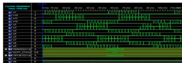
Figure: 17 Gate pulse generated from FPGA for 7 level inverter voltages.
